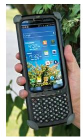
in cradle with spare battery charger may be used for desk-top or vehicle mounting. The device is IP67 rated and meets or exceeds MIL-STD 810G using methods 516.6 and method 514.6 for both shock and vibration.
