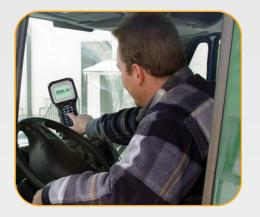
ing, load management, real time asset tracking, electronic DOT and fuel tax data collection, LoadTrek.net incorporates Two Technologies' JETT® • ce rugged, handheld computers as the onboard interface for communicating information between the truck's onboard computer, the driver and the home office.
